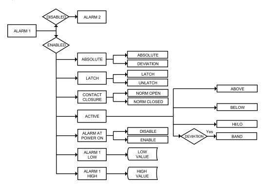
Figure 3.5 Flow Chart for Alarm 1
